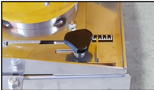
SHUTTER STOP PLATE CLOSED (Setting 0)
